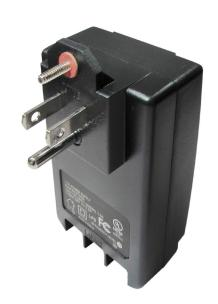
The OE-PPS12V1AS is a fully regulated 12VDC, 1 amp plug-in switching adapter that provides reliable DC power for a wide variety of indoor security and surveillance products and applications. It can be used with input voltage ranging from 100 to 240VAC and includes a power indicator LED. Self-limiting protection against short circuit and overload conditions is included, with auto recovery. Complies with DOE Level VI Efficiency and FCC requirements.
